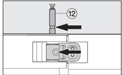
■ Push hinge pin ⑫ in until the groove on the pin is in line with the drill holes in the bearing block.
